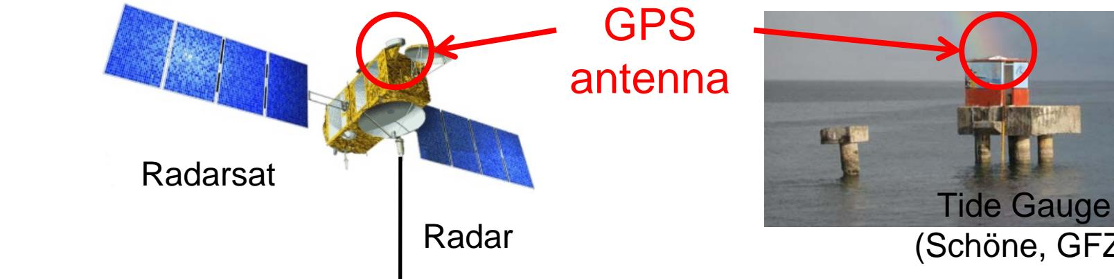
Precise satellite and ground station GPS processing for sea level measurements at GFZ
